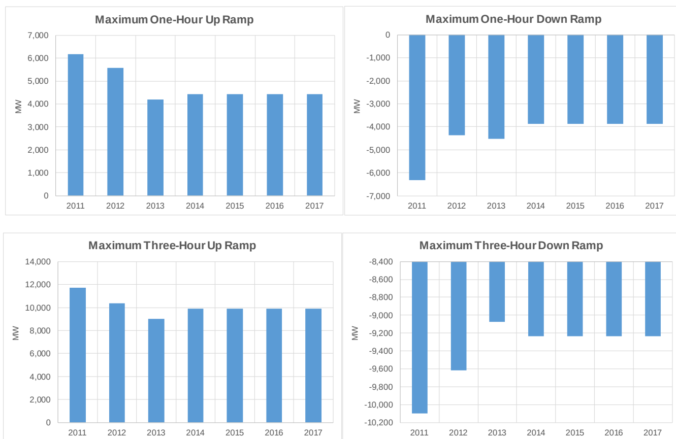
Figure B.18: Southern Company maximum 1- and 3-hour net load up and down ramps
